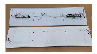
Pictured 2 row configuration with drivers installed. Front and back
